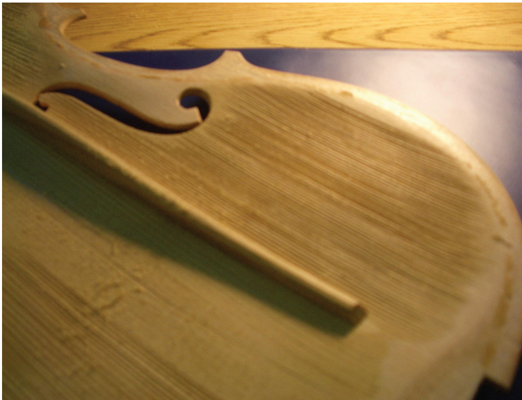
Figure 4. Riffled spruce violin top with untouched center section.
