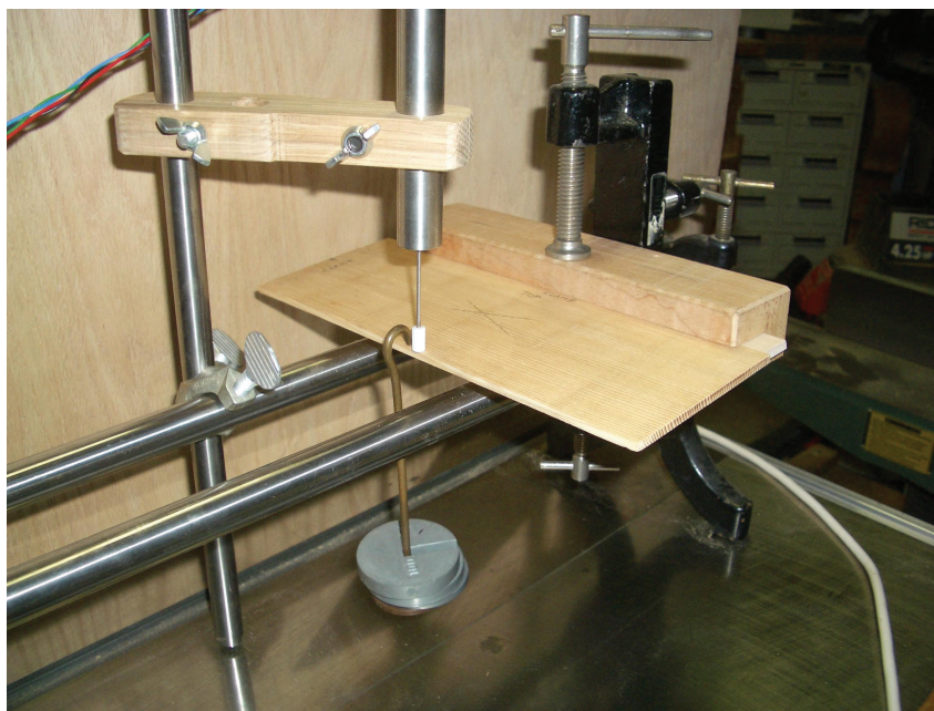
Figure 1. Load-deflection measurement of a spruce plate perpendicular to the grain. A linear variable differential transformer (LVDT) is used for measurement of displacement.
