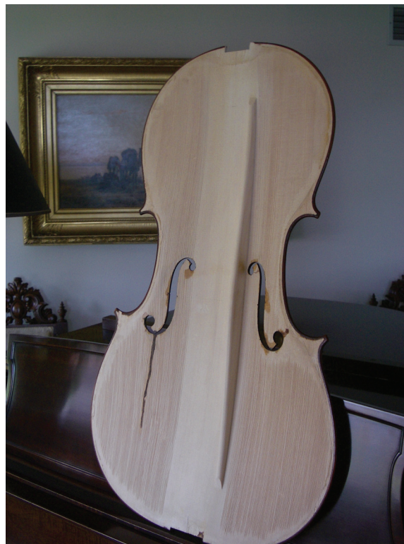
Figure 7. Riffled spruce cello top with untouched center section.
