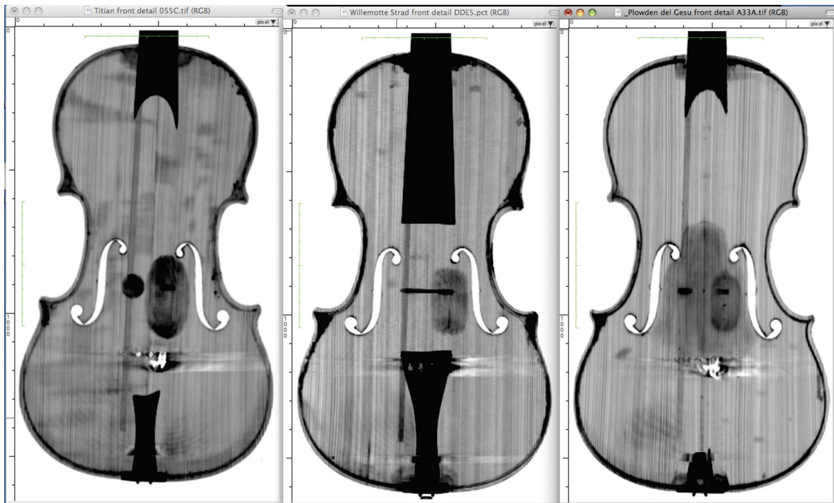
Figure 4. CT measured images of the spruce tops of the three Old Italian violins. Left to right are the Titian Stradivari (1715), the Willemotte Stradivari (1734), and the Plowden Guarneri del Gesù (1735). (See Figs. 34-36 for CT density profiles extracted from these CT scans.)
