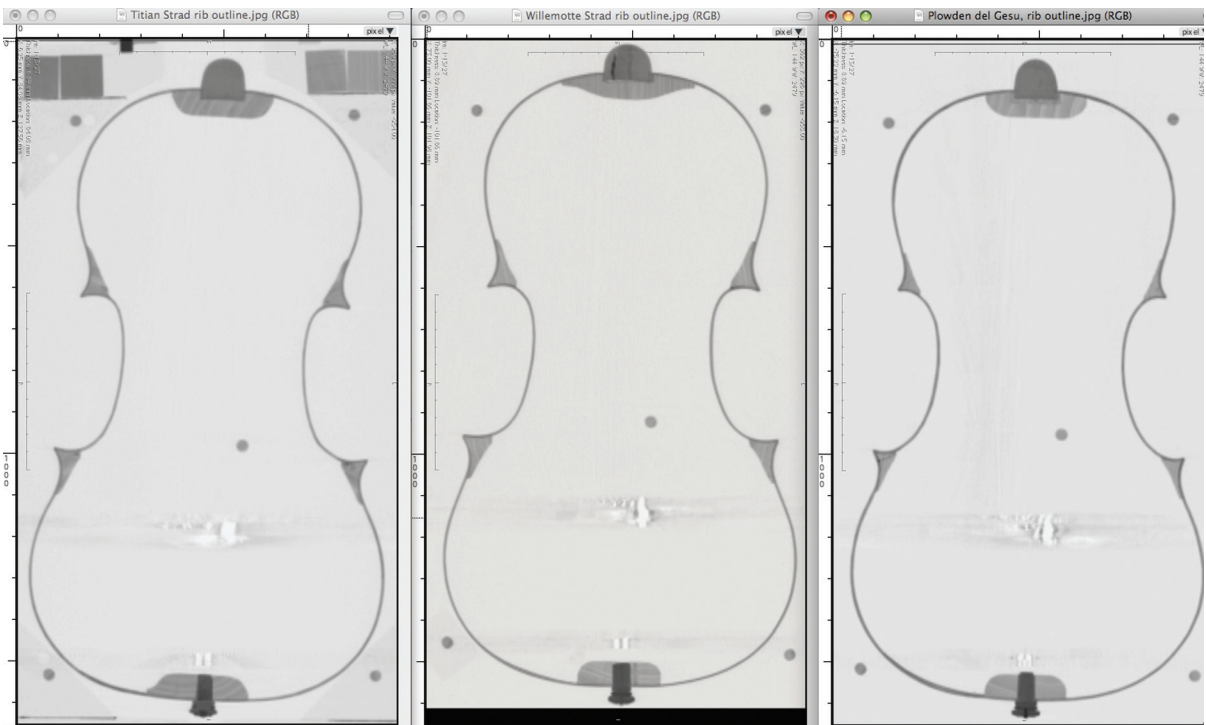
Figure 5. CT images of the rib outlines of the three Old Italian violins. Left to right are the Titian Stradivari (1715), the Willemotte Stradivari (1734), and the Plowden Guarneri del Gesù (1735).
