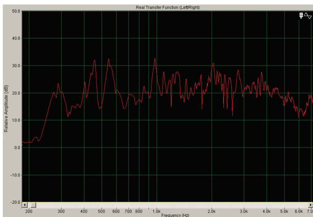
Figure 7. Sound spectrum radiated from the Titian Stradivari violin. The test configuration was the same as in Fig. 6.
