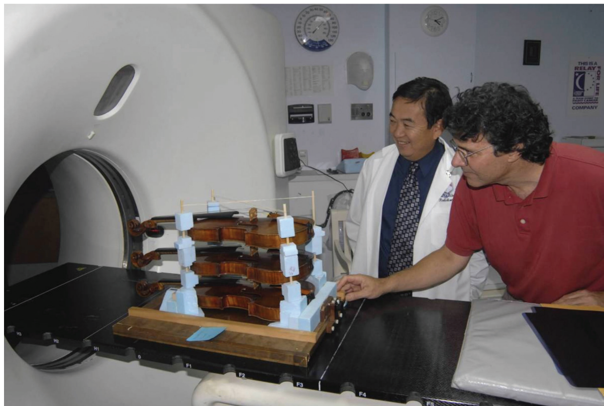
Figure 2. With the Old Italian violins stacked three high ("Cremona sandwich"), Dr. Claudio Sibata, head of the medical physics staff of the Leo Jenkins Cancer Center (East Carolina University), performed the x-ray CT scans. Sam Zygmuntowicz is shown assisting.
